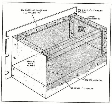
Fig. 3. If chassis supporting brackets are not used special side plates made of aluminum can be used. Copper screening would then be necessary only for top and back.
