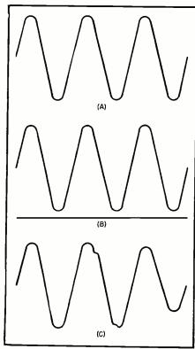
Fig. 2. Patterns observed when line is incorrectly terminated. (A) Phasing adjustment on sweep generator correctly set. (B) Sweep generator blanked during return sweep. (C) Pattern resulting when there is a fault on the line.
