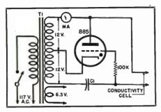
Fig. 5. Phase-sensitive conductivity bridge.  $C_1$  is determined by the probe and solution characteristics. It may range from .001 to 10 mfd.
