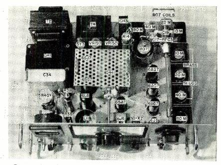
Top view of the v.f.o.-exciter unit shows location of the major circuit components.
