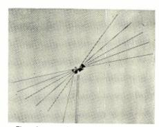
Fig. 13. Broadband response obtained by a "fan" of dipole elements.
