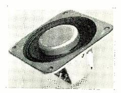
An aluminum cup driven by a loudspeaker at 60 cycles is used as a mechanical inductive sweep. This cup is located near the tank coil of the master variable oscillator. Thus, the actual inductance of this coil is varied and with it the frequency. Photo below shows position of speaker on chassis.
