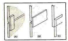
Fig. 5. A good overlap on trap doors is important. An opening like that shown in (A) spoils the shielding. While (B) is much better than that shown in (A), (C) is preferred, providing better shielding.
