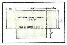
Fig. 4. Details for cutting wire screening.
