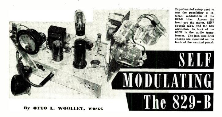
A novel method of using a single 829-B as an r.f. amplifier and modulator. The common cathode and screen are modulated.
