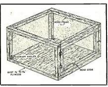
Fig. 7. A wooden framework completely covered on six sides with copper screening can be used to shield entire unit.
