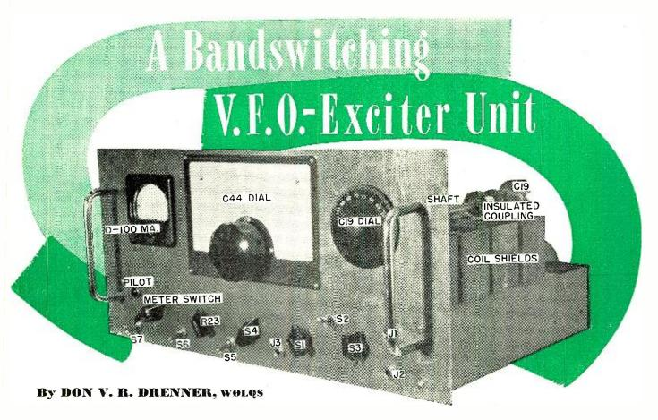
Construction details on a v.f.o. exciter with output on the 10, 20, 40, and 80 meter ham bands.
