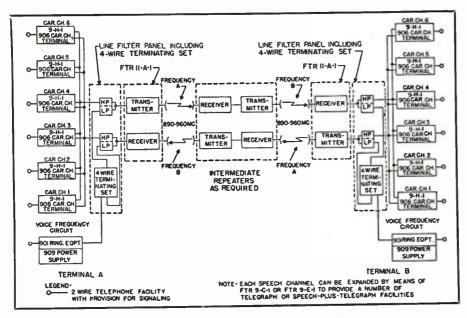
Fig. 3. Detailed block diagram of 7-channel two-way link system.
