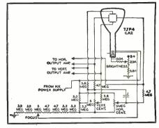
Fig. 9. Method of applying the high accelerating voltage to the image tube and also providing beam centering adjustments.
