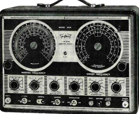
Two Built-in Markers Can Be **Used Simultaneously Giving** Facilities for Faster Identification of Bandpass of Curves Without Constant Tuning of Marker
