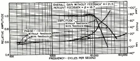
Fig. 2. Steady-state response measurements of an amplifier with and without feedback.
