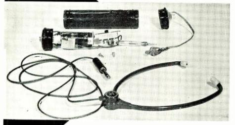
Left, assembled, and right, disassembled view of tracer.
