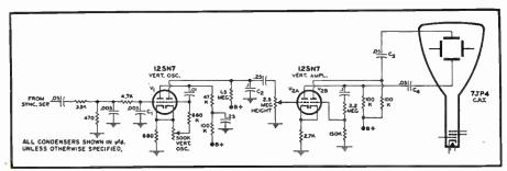
Fig. 2. A widely-used vertical sweep system.
