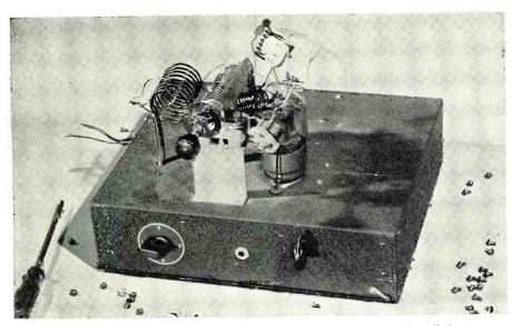
This is a 28 mc. 815 "breadboard" type with 56 mc. plate traps installed.
