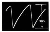
Fig. 4. The proper method of presenting a saw-tooth wave, with its amplitude indicated, in the receiver service manual.
