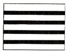
Fig. 2. Number of dark horizontal bars caused by heavy oscillations in the camera chain. In this case the trouble was due to a poor connection in a heater transformer. Resoldering the defective connection corrected the trouble.
