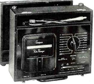
In the Simpson "Roto Ranger," proper meter scale automatically comes into view as the range selector switch is turned. This feature facilitates rapid reading of the meter needle. Sensitivity is 20,000 ohms. per-volt, and 25 voltage, current, and resistance ranges are available. Meter is in size. Price is approximately \$70.
