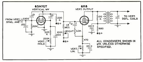
Fig. 8. A vertical deflection system feeding  $\alpha$  set of deflection coils.
