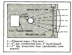
Fig. 4. Light source assembly. Unit contains the light, infrared filter, projection lens, and a filament transformer.
