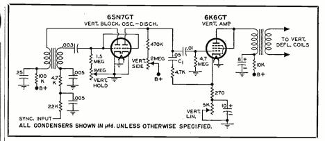
Fig. 13. A vertical sweep system using a blocking oscillator.
