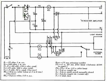
Fig. 3. Wiring diagram of the indicator-control assembly.
