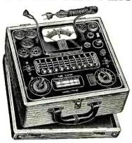
The Model TV-10 operates on 105-130 Volt 60 cycles A.C. Comes housed in a \$950 beautiful hand-rubbed oak cabinet complete with portable
