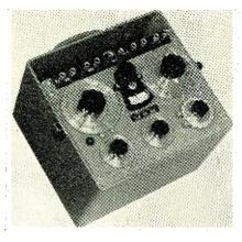
capacitance, and inductance over the following ranges: Resistance, 1 milliohm to 1 megohm; capacitance, 1 μμfd. to 100 µfd.; inductance, 1 µhy. to 100 hy. It is enclosed in a  $9\frac{1}{2}$  by  $10\frac{1}{2}$  inch cast aluminum cabinet and is powered by four replaceable flashlight cells.
