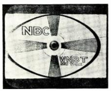
Fig. 5. Image possessing insufficient height.
