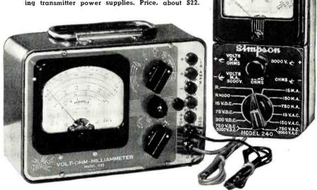
The four-inch meter dominates the case of the Hickok Model 435 volt-ohm-milliammeter, with 35 ranges, a sensitivity of 20,000 ohms-per-volt, and d.c. and a.c. power supplies. Price of unit is about \$38.
