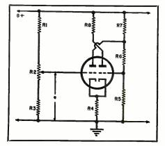
Fig. 1. Basic Schmitt trigger circuit.  $V_1$  is the left half and  $V_2$  is the right half of the dual triode.
