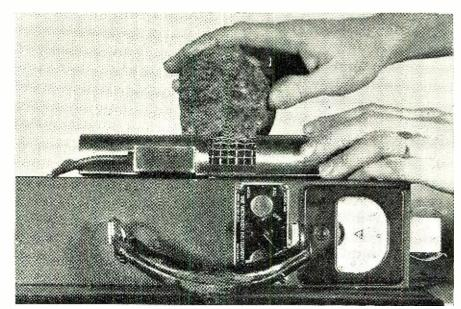
Fig. 3. Measuring mineral radioactivity. When screen mesh is exposed, beta, gamma, and higher radiations will be detected. When screen is shielded by metal slide, beta component will not be detected. It can be used in field exploration work.
