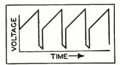
Fig. 10. The proper deflection voltage to use with deflection coils.
