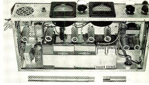
A view of the electronic unit removed from the cable drum.
