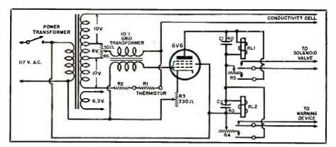
Fig. 2. Complete circuit diagram of the conductivity bridge.
