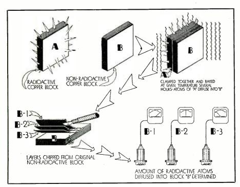
Fig. 1. Self-diffusion technique, imparting radioactivity to pieces of like materal, then measuring chips for presence of radioactivity with Geiger-Mueller detectors.
