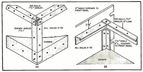
bent to form the angles. In the case of galvanized iron or copper, it may be soldered together or assembled with machine screws and nuts as this material is too thin for tapping. Flat strips of brass may be used in place of the angles if they are easier to obtain. These should be from  $\frac{3}{16}$  to  $\frac{1}{8}$  inch thick and  $\frac{3}{4}$  to 1 inch wide for rigidity. Also the dimensions should be altered to fit the particular chassis and panel size used.
