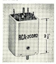
amplifier of television receivers to attenuate the 4.5 megacycle intercarrier beat frequency. The design utilizes a fixed, ceramic capacitor shunting a low-Q inductance tuned by an adjustable iron core.
