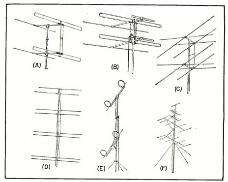
Fig. 16. Several types of commercially available stacked arrays that provide a higher gain and an improved directional pattern.
