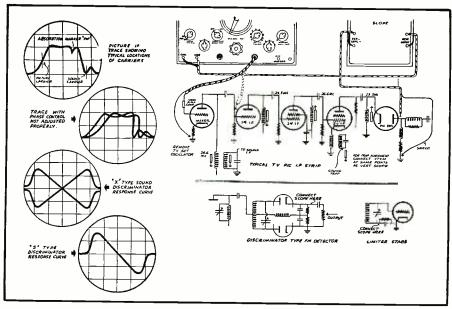
Fig. 1. A sketch showing a few of the many uses of a properly designed sweep generator when used in visual alignment techniques.
