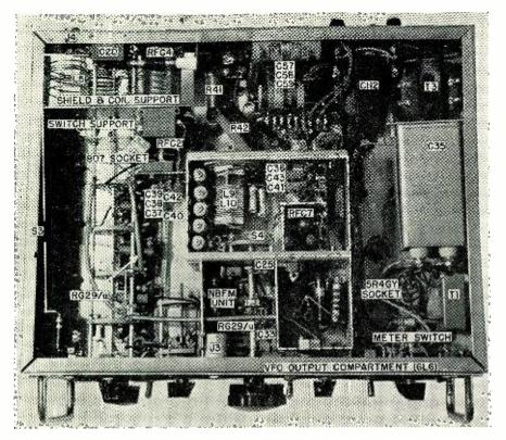
Under chassis view. The oscillator and NBFM portions are enclosed in box shields.
