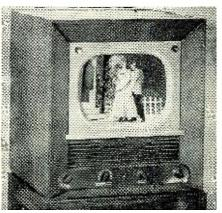
table is the first receiver made by General Electric, Syracuse, N. Y., to use a 16-inch picture tube. Appearing to be one piece of furniture, the ensemble retains the convenience of separate units.
