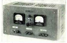
rents from 0 to 200 milliamperes, regulated; a.c. output is 6.3 volts at 6 amperes, unregulated.
