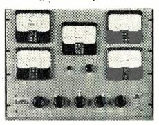
currents in the several elements of the array. Phase indication is clearly displayed on a meter marked in two-degree intervals.
