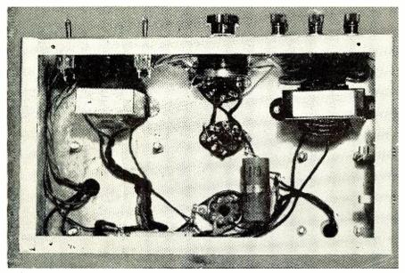
Fig. 4. The two meter jacks are mounted through this end of the chassis. The voltmeter plug, for reading d.c. output voltage, is shown inserted into its jack.
