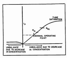
Fig. 4. Plate current of detecting tube.
