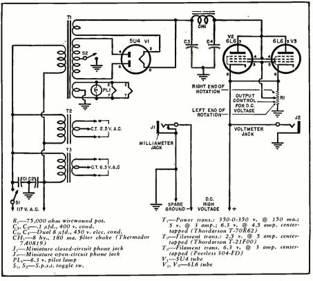
Fig. 2. Complete wiring diagram of the experimenter's low-cost power supply.
