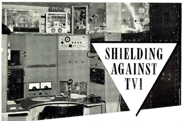
On top of the relay racks may be seen several breadboard units that have been properly shielded. All r.f. units in the cabinets have been shielded similarly to the 829 unit described in the article.
